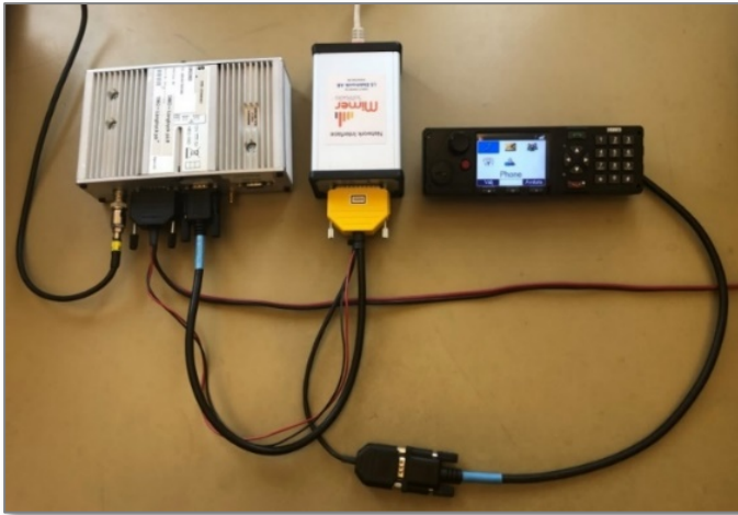
Sepura SRG with Network Interface and cable kit The connections are the same on the SCG22
