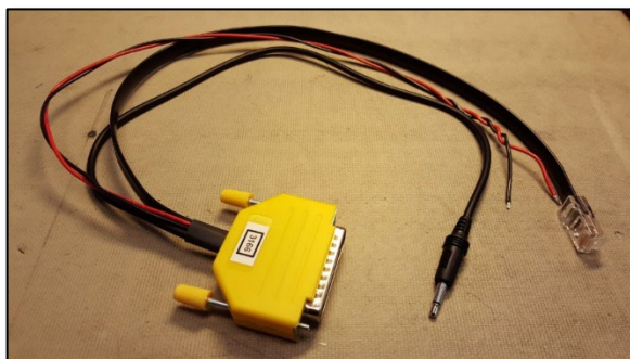
Cable Kit 3166/02 for Icom IC-A120
