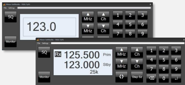
Virtual Control Heads of Trig TY91
