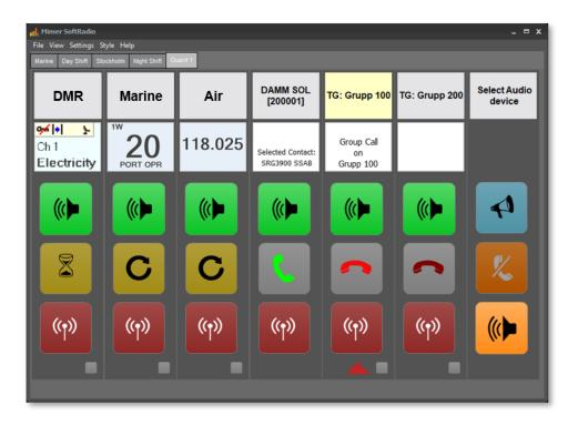
Example of SoftRadio with three radios (DMR, Marine and Airband) and one Tetra system with two talkgroups attached
