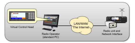
A radio connected to an operator PC
