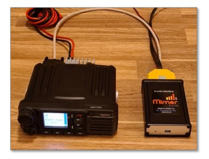
Hytera MD785 connected to a X-Link interface
