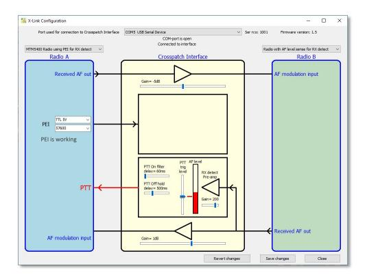
In this illustration the AF level is above the PTT trig level and a PTT command is sent to the other radio
