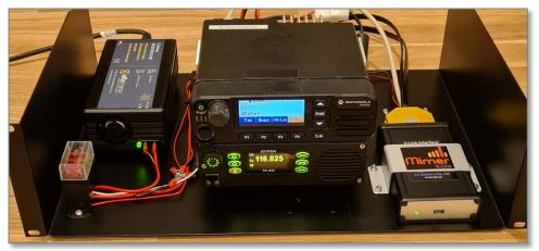
Jotron TR810 installed together with a MotoTrbo radio and the X-Link interface on a rack shelf.
