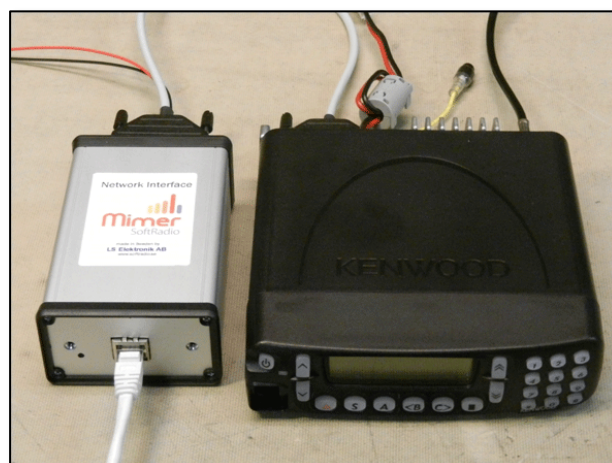
Network Interface connected to Kenwood TK-8189
