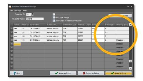
Example with three radios all working on CH16, connected in one diversity group.
