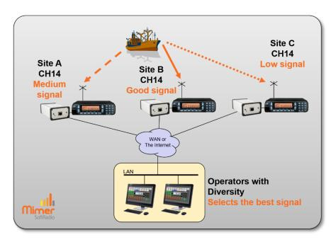
Example of system with three base stations on CH14 and the ship travelling between the radios coverage areas.
