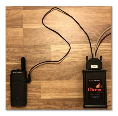
Cable kit X-Link to Motorola portable
