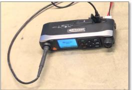
Cable kit X-Link to Kirisun and connections to the radio
