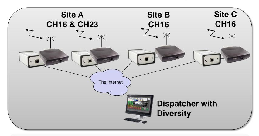
In systems with several base stations on the same channel these can be connected together in a voting system so the operator always gets the best audio
