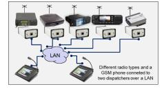
The SoftRadio systems does not have a Central Controller. All intelligence is in the network interfaces and in the operator software.
