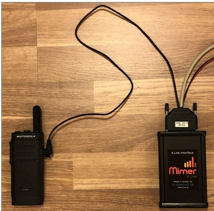
*Cable kit X-Link to Motorola portable*
