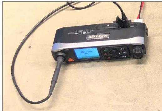
*Cable kit X-Link to Kirisun and connections to the radio*
