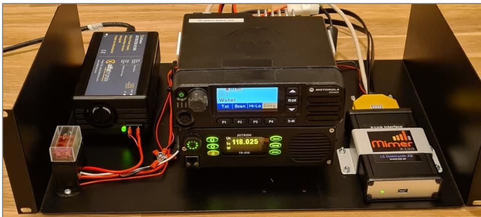
*Jotron TR810 installed together with a MotoTrbo radio and the X-Link interface on a rack shelf.*
