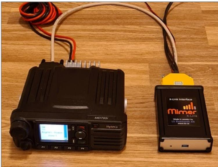
*Hytera MD785 connected to a X-Link interface*
