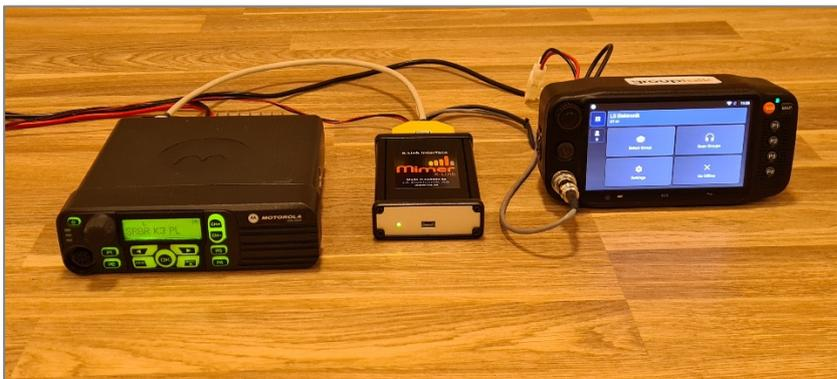
*Radio connected through X-Link to Estalky*
