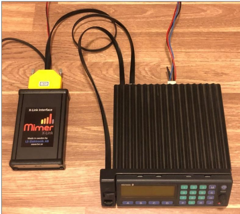
*Cable kit X-Link to Aurora mobile, connected in the back*
