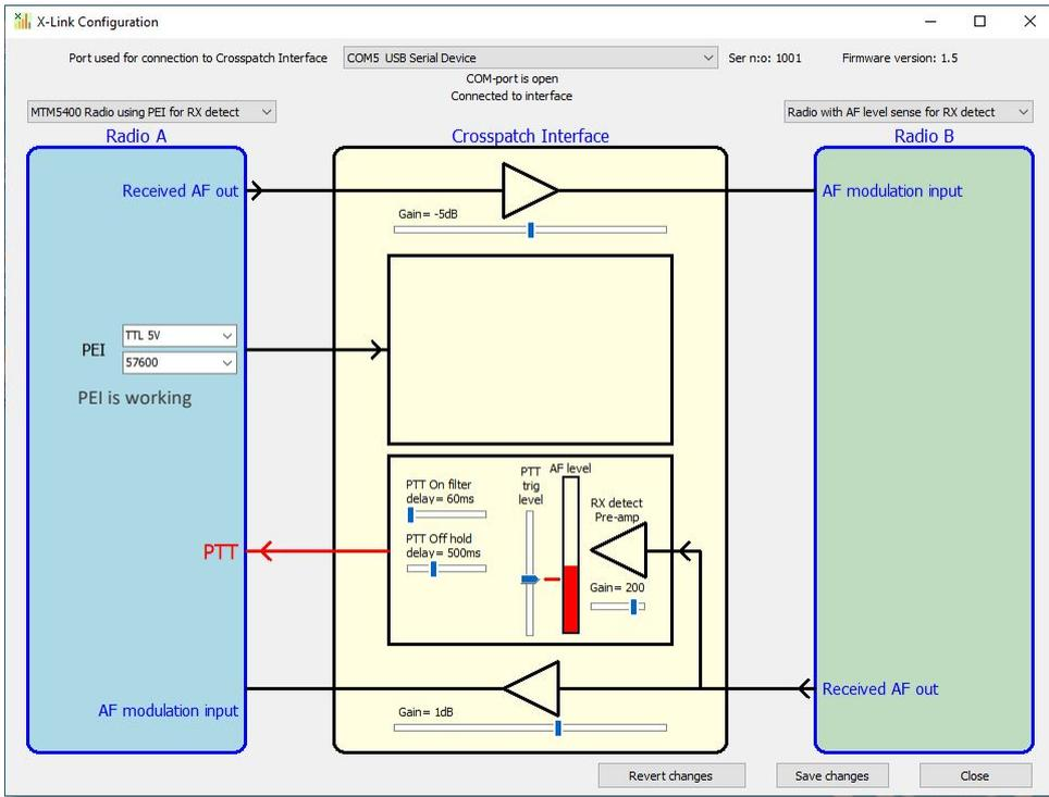
*In this illustration the AF level is above the PTT trig level and a PTT command is sent to the other radio*
