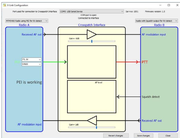
In the picture above, Radio A is receiving (green arrow) and the interface is giving Radio B a PTT signal (red arrow).
