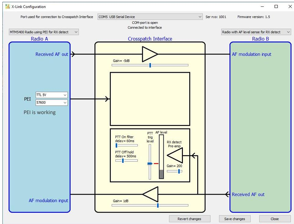
*In this illustration the AF level is below the PTT trig level and no PTT command is sent*
