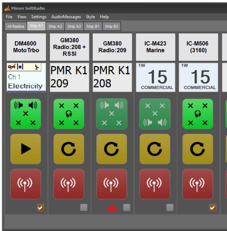
*In the example above the first radio is monitored in the two front speakers. The second radio is monitored in the headset. The third radio is not monitored at all, and so on.*
