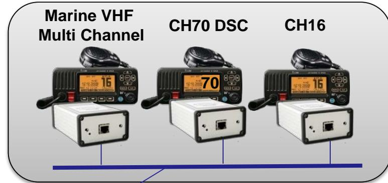
Typical marine setup with fixed radios for CH16 and CH70(DSC) at each site.
