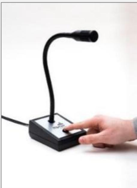
This is the basic microphone with PTT. It connects to the PC's analogue microphone port and with a separate cable to the COM-port for the PTT function. If your PC doesn't have a COM-port, a USB dongle can be used.
