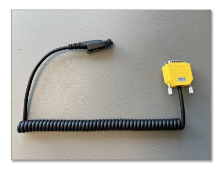
(Picture showing cable for X-Link, with the smaller D-sub)
