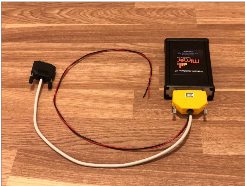
Cable kit connected to NetworkInterface LE
