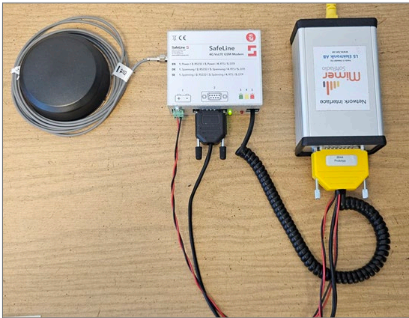
Phone module together with network interface
