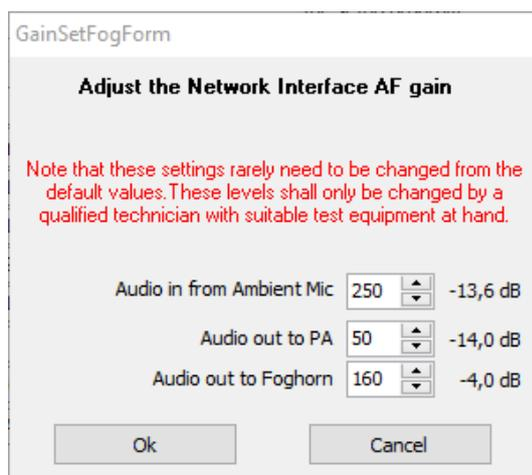
The maximum gain for PA and FogHorn are 0dB, represented by a value of 255. Normally you would like the FogHorn to be louder than the PA speaker and therefore it is set to a higher value.
