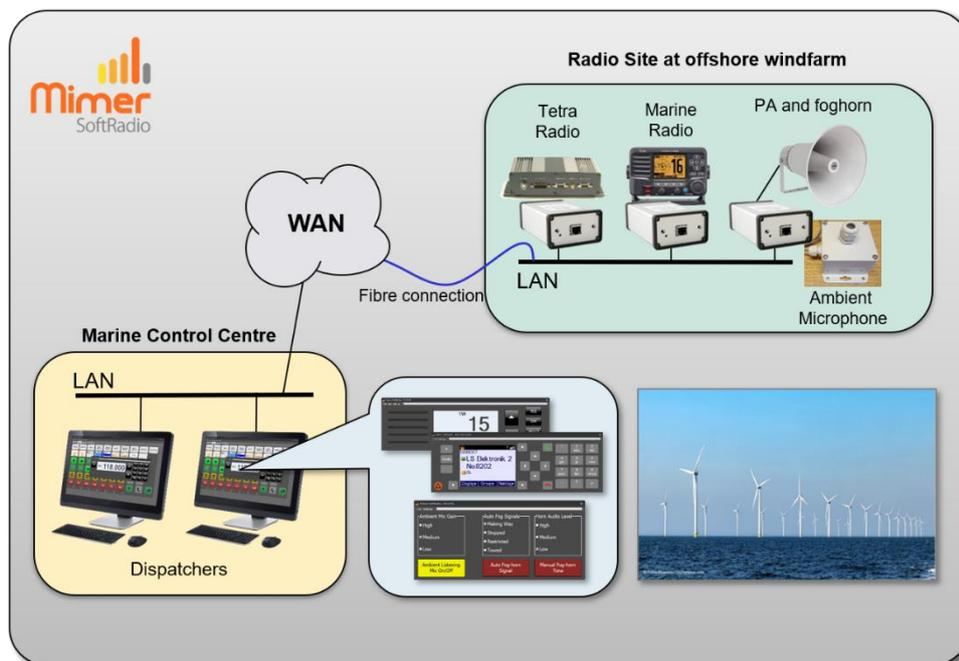
*Example of windfarm system with two operators working with two radios and an interface for PA, fog horn signalling and ambient listening.*
