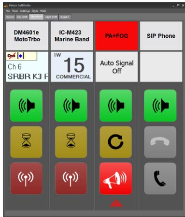
*Mimer SoftRadio with two radios, a phone and a PA & FogHorn unit connected. The operator is talking on the PA speaker.*
