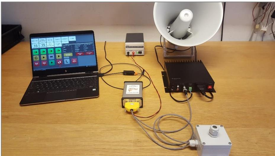
*Test setup with SoftRadio on a laptop, local network to the interface, microphone and amplifier/speaker.*
